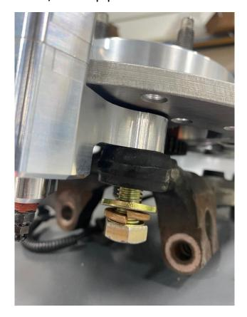
\*Drop the pads into the calipers with the friction side facing the rotor and secure them with the pad retaining bolt and ny-lock nut. Be sure the bolt extends through the locking feature of the nut and tighten until you can barely spin the pad bolt with your fingers. Make sure the brake pads are the only thing touching the rotor! The rotor should be centered in the caliper.
