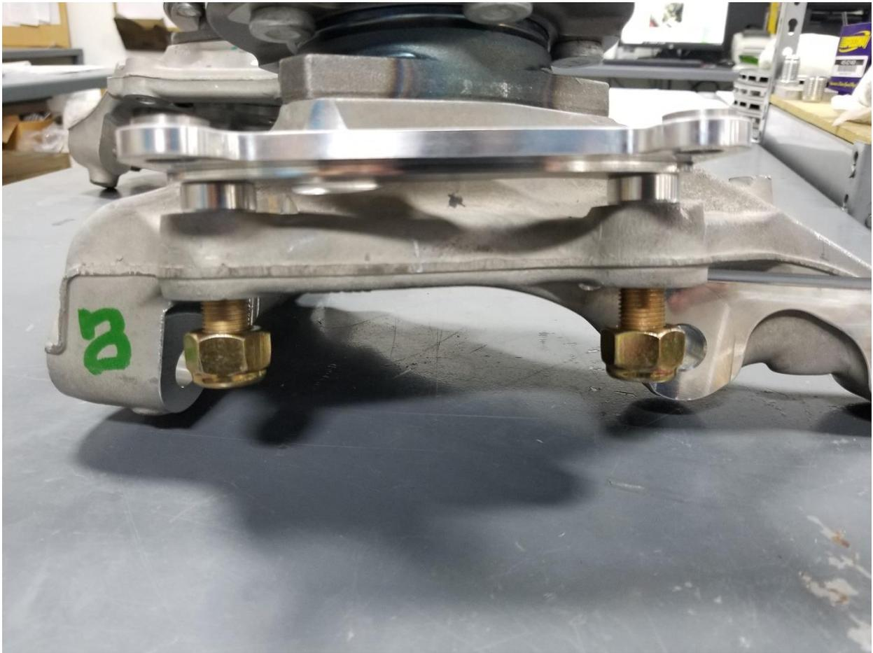
\*Bolt rotors to hats using the 5/16 -18  $\frac{3}{4}$  low head screws. Make sure to clean bolts with acetone and use red Loctite to secure. The hat should be mounted on the flat side of the rotor.
